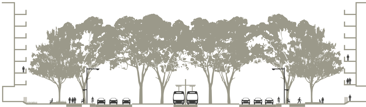
FIGURE 15: Formal landscape avenue cross-section medium term Northbourne Avenue 3 lanes each way with protected cycle lane
