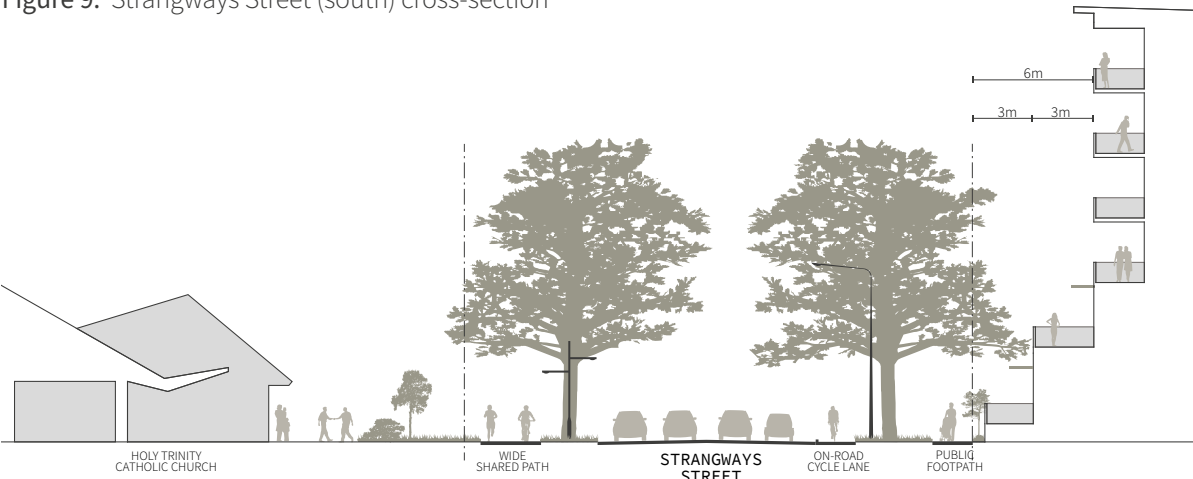
Figure 9: Strangways Street (south) cross-section
