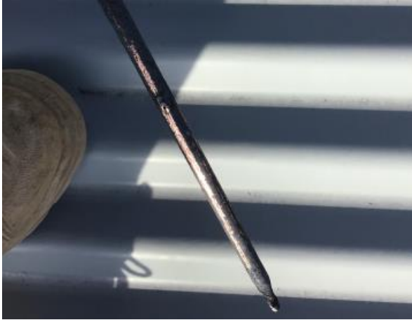
Figure 6: Example of split copper heat pipe in solar evacuated tube
