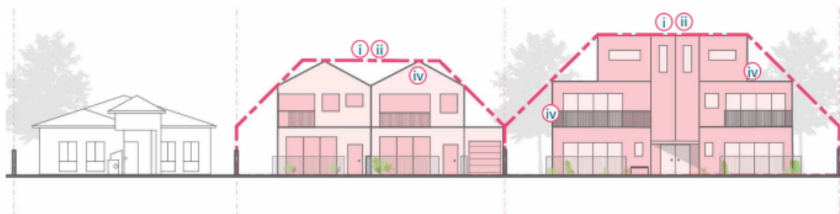
Figure 45: Larger block widths and depths enable a greater building envelope while maintaining a consistent neighbourhood feel and character.
