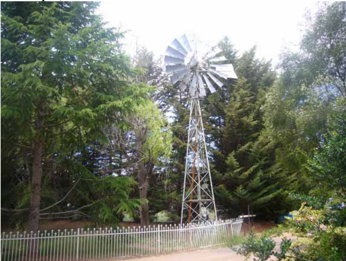
Figure 29. Windmill used to operate the water pump that replenishes the small pond.
