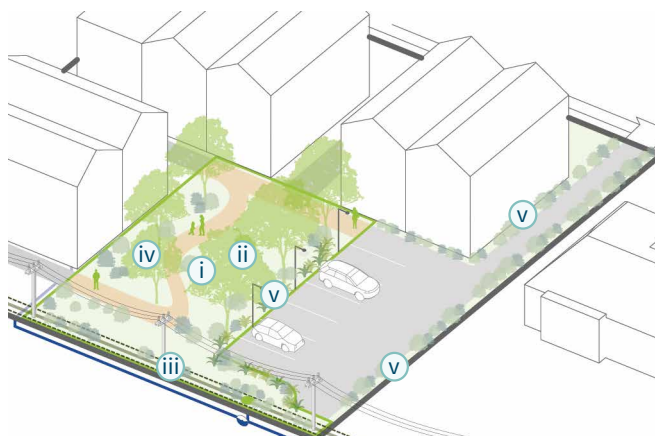
Figure 97: Landscaping should maximise planting areas and tree canopy while avoiding areas required for hardscaping and easement maintenance.
