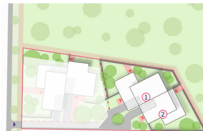
Figure 14: Dual-occupancy on a 'battle-axe' block with frontage to a public open space. The buildings are positioned to allow for front gardens and direct access to the public open space. This supports the activation and passive surveillance to the public open space.
