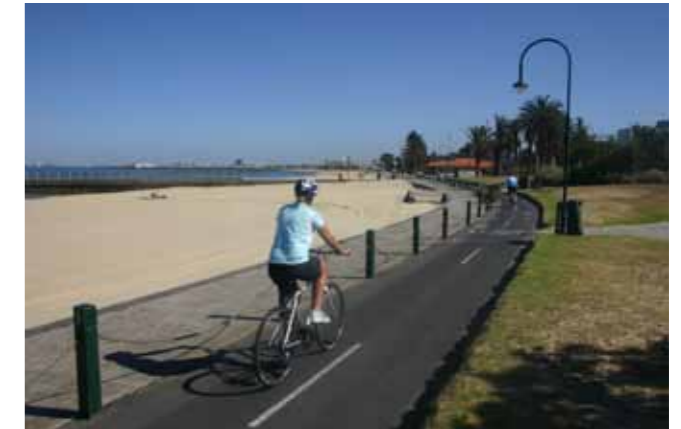
Figure 11 – Cyclists and pedestrians are separated by fencing and contrasting surface.
