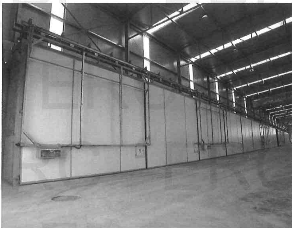
Figure 7: Example of a composting tunnel, external view. Image supplied by technology composting provider Christiaens
