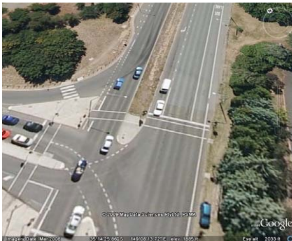
Northbourne Avenue at Barton Highway showing the Bus lane and B Light allowing buses to cross the intersection ahead of queuing traffic.
