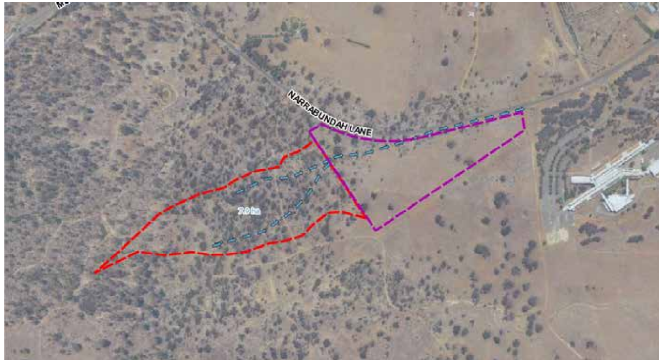
Figure 11: Existing flow paths through the potential mental health site
