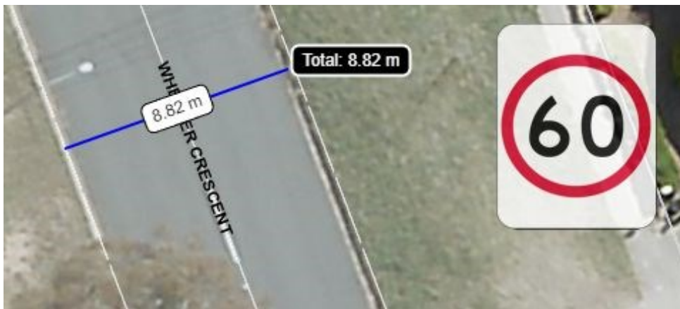
Figure 19: Wheeler Crescent has a 60 km/h speed limit for its entire length, but also has traffic calming installed in many sections. Why advise motorists they can safely travel at 60 km/h, then install traffic calming which requires them to routinely slow to 20 km/h? That doesn't make sense. Wheeler Crescent is also 9 metres wide for almost its entire length. Why is this road set at 60 km/h, but Longmore Cres and Langdon Avenue, roads that are almost identical in width and purpose, have 50 km/h speed limits?
