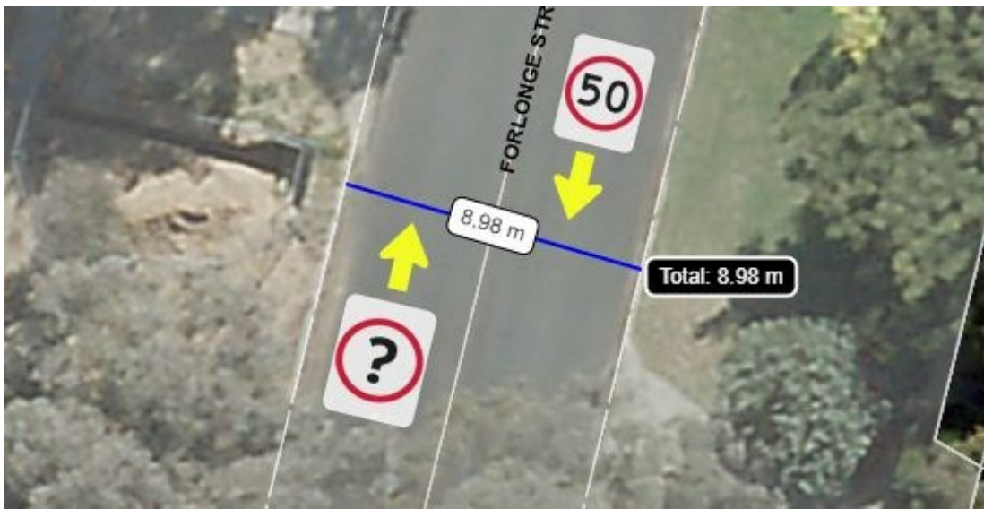
Figure 7: Image of Forlonge Street between Taverner Street and Fincham Crescent. Motorists who enter Forlonge Street from Taverner Street will pass two 60 km/h signs, but those entering the same street from Wheeler Crescent will not pass any signs. For motorists travelling Northbound on Forlonge Street, two speed limits can apply to the same length of road in the same direction. Motorists travelling southbound have not passed any signs by this point, so must obey a 50 km/h speed limit.
